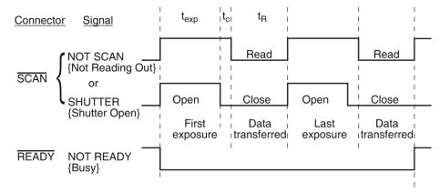
Figure 37. Comparison of NOT SCAN {Not Reading Out}, SHUTTER {Shutter Open}, and NOT READY {Busy} Logic Output Levels
